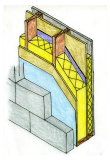
The combined protection provided by the vapour barrier (internally) and the breather membrane (externally) ensures the timber inner leaf remains dry at all times.
