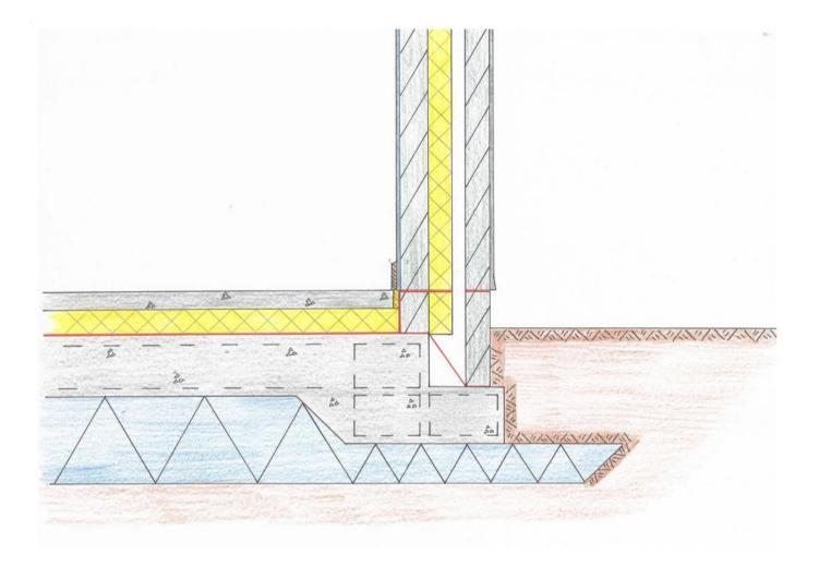
The concrete raft is supported on a compacted hardcore base which extends out past the edge of the raft.
