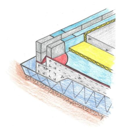
100mm of rigid insulation is installed below the finished floor to ensure that there is no heat lost through the foundation.
