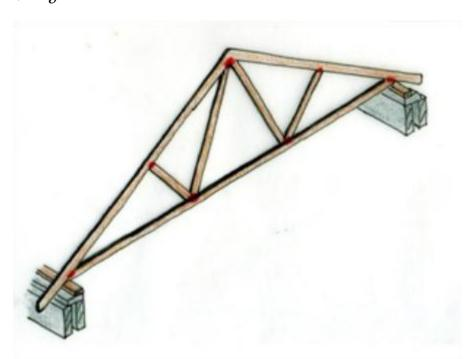
Each truss is delivered to site and they are then attached to the wallplate and placed at 400mm centres.
