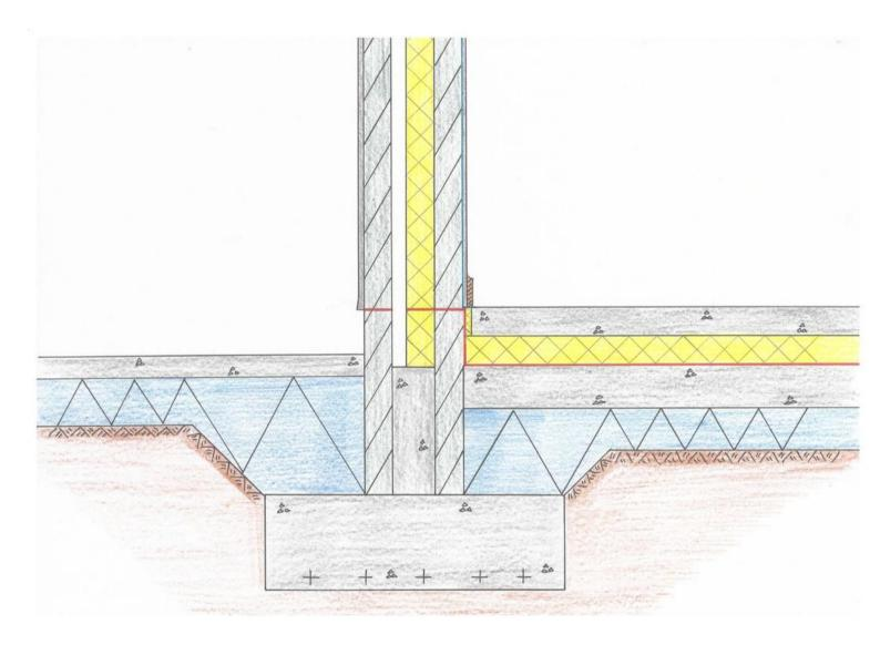
The size and position of a concrete strip foundation is directly related to the overall width of the wall.
