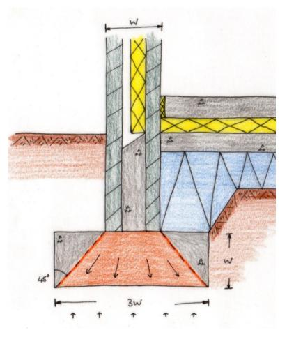
It is vital that the strip foundation is strengthened through the inclusion of steel reinforcement.
