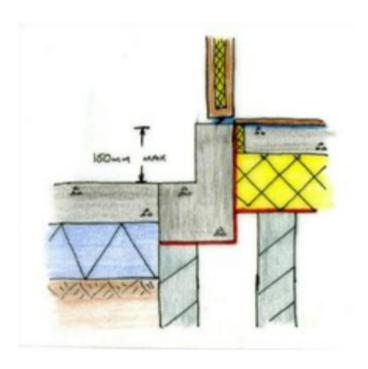
There is also a stepped alternative for the threshold detail.
