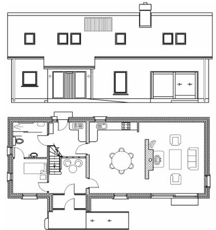
7. A new extension has been constructed to a dormer bungalow to provide space for a new kitchen area as shown in the sketch. The new extension has a solid concrete floor with a tiled finish. The existing bungalow was constructed with a 350 mm insulated cavity wall and has a suspended timber floor.
