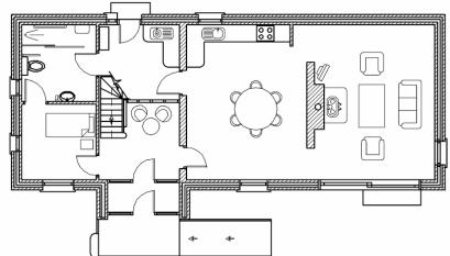
7. A new extension has been constructed to a dormer bungalow to provide space for a new kitchen area as shown in the sketch. The new extension has a solid concrete floor with a tiled finish. The existing bungalow was constructed with a 350 mm insulated cavity wall and has a suspended timber floor.
