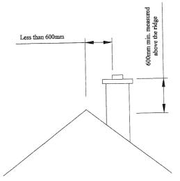
chimney should be a minimum of 1 metre above the highest point of contact with the roof slope if the chimney is 600 mm or more away from the ridge // chimney should be a minimum of 600 mm above the ridge if less than 60 mm
