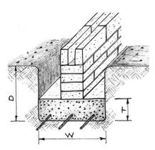
the depth of the foundation (D) depends on soil type and weight of the structure to
