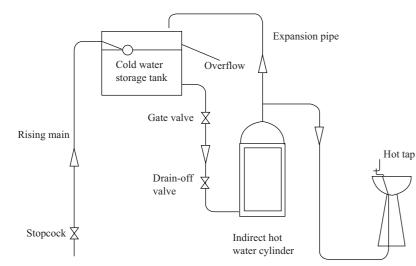
**(b)** Show, using notes and neat freehand sketches, one design detail that should be used to prevent heat loss in the hot water system. (10m)
