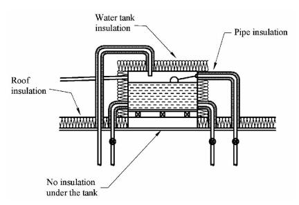
**(b)** Include in your sketch **two** design details that would prevent the water in the storage tank from freezing during very cold weather.
